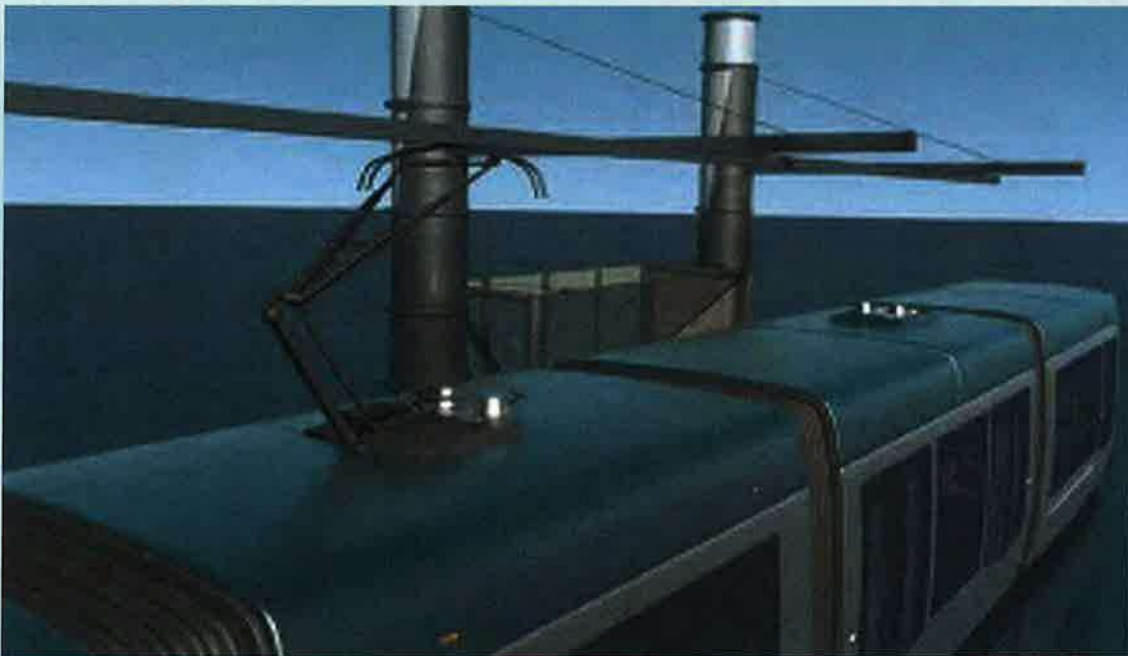
Short Rigid OCS at Station Stops. Courtesy of CAF
