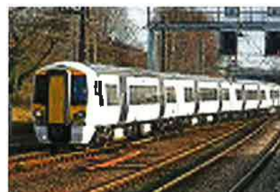
Test Electrostar Train converted to run on batteries and overhead wires
