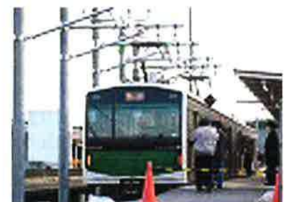
EV-E301 charging from the overhead conductor bar
