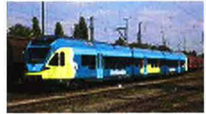
Stadler FLIRT Akku battery train, to be trialled in Denmark
